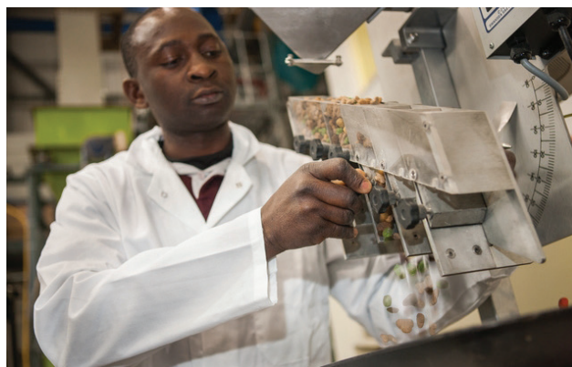
Evaluation of segregation behaviour (surface or air effect) can be undertaken using unique testing equipment
